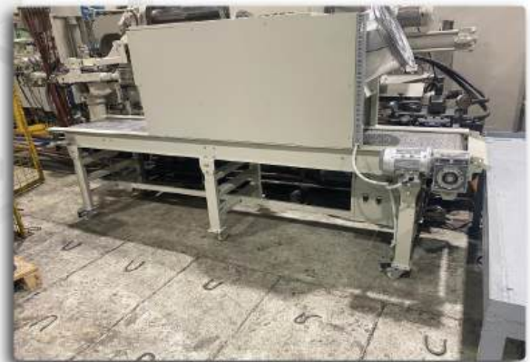
Stainless steel chain conveyor system for zinc casting workshop
