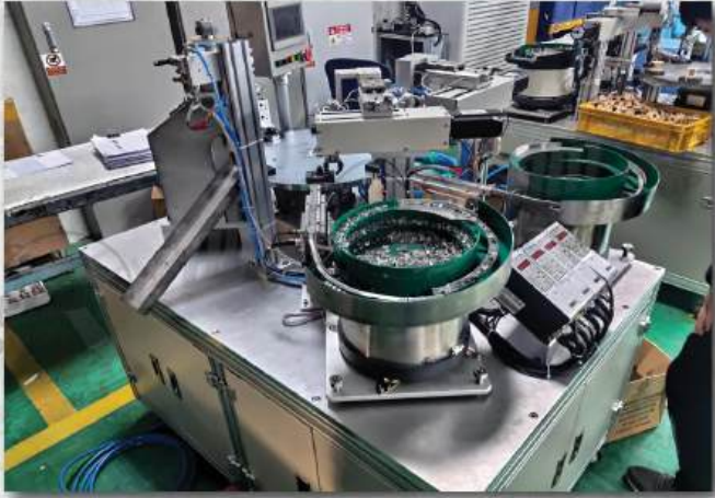
Automatic motor assembly machine for vacuum cleaners, replacing 6 operators.
